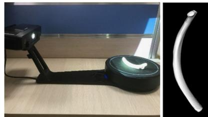
Fig. 14. 3-D scanner used to collect the 3-D model of ribs.
